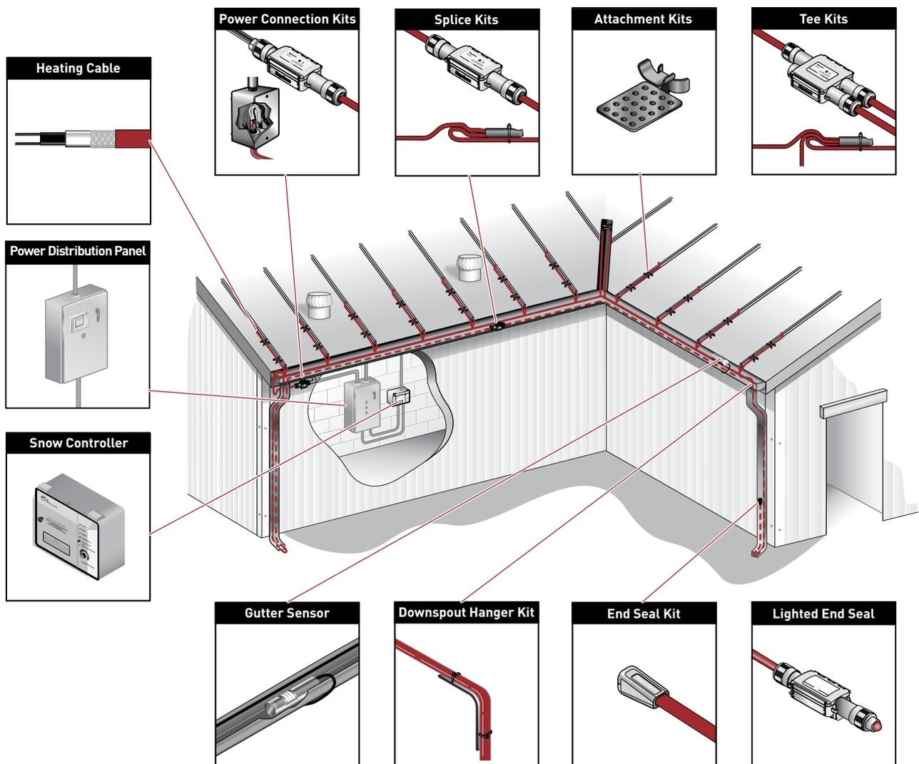
Fig. 1 Typical IceStop roof and gutter de-icing system
