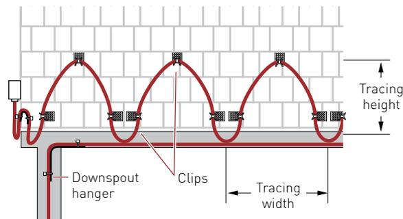
**Fig. 5 Front view of roof with IceStop system**
