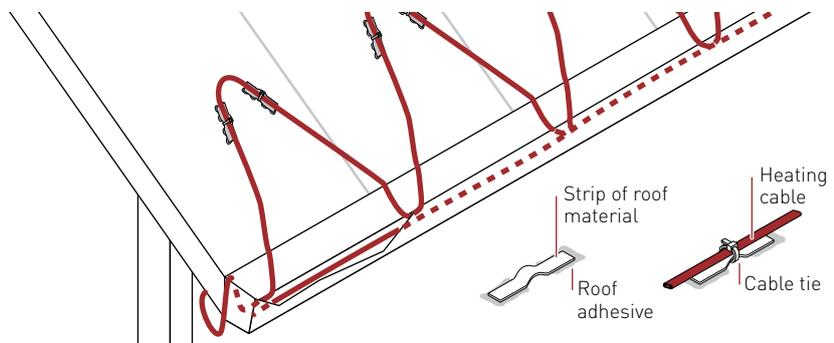
**Fig. 21 Belt loop approach on a sloped roof**
