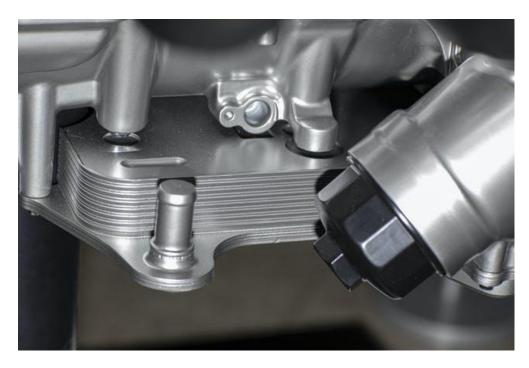
Being the largest flat-plane V-8 in production means that there will be inevitable vibrations. Having a light rotating and reciprocating assembly will reduce the severity of these vibrations, but at some point, as Gartner put it, "you have to tolerate it." A low-torque, spin-on oil filter canister is in danger of vibrating itself loose on an engine like this, so Chevrolet opted for a cartridge-style oil filter for the LT6.
