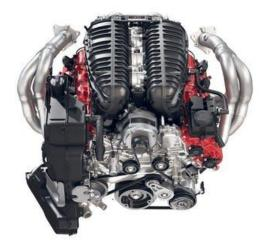
A flat-plane crank removes a lot of mass, somewhere in the range of 30 to 40 percent compared to a cross-plane unit. According to Gartner, the aluminum, viscous-filled front damper on the LT6, is also "drastically lighter" than an iron elastomer damper like the one found on the LT2. The rear flywheel-side damper is similar to the one on the LT2 but is also lighter.
