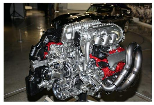
While the car will likely have a suggested 500-mile break-in period before it should be subjected to any all-out track shenanigans, the engine will already have a 20-minute dyno break-in where it's warmed up and put through its paces and finally run at 7600-rpm for a WOT pull.
