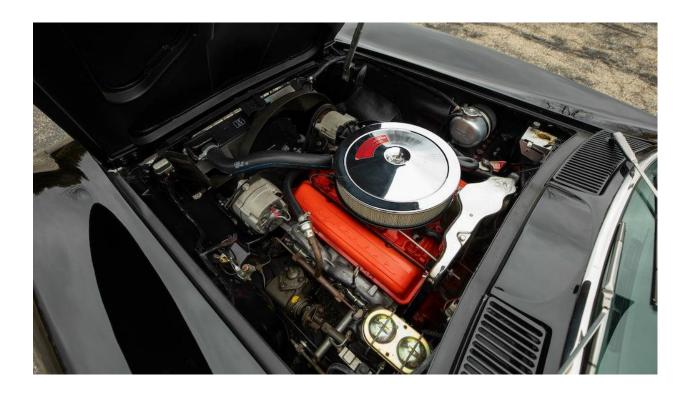
This particular 1967 Corvette is powered by GM's 327 cubic-inch small block V8, originally rated to produce 300 horsepower, which flows to the wheels via a Muncie M20 four-speed manual gearbox and Positraction rear end. The C2 rolls on a nice-looking set of Rally wheels wrapped with BF Goodrich 7.75×15 Silvertown Redline tires, helping to retain its OEM factory goodness.
